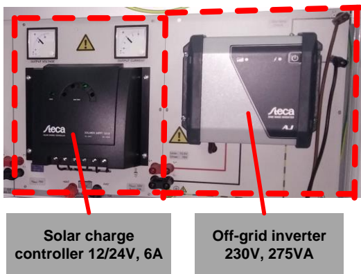
Figure 6. Solar charge controller and Off-grid inverter
